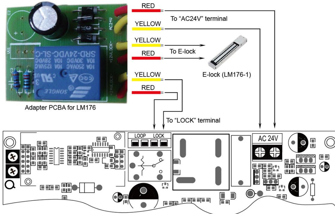
**Note: The polarity of the wires can not be connected by mistake to avoid damaging the components.**
